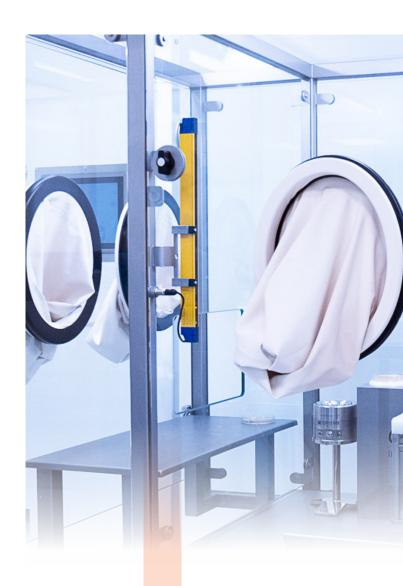
The ISO class 6 area is fitted with a filling line under a Laminar Air Flow unit to generate an ISO class 5 environment for aseptic filling of vials and syringes.
