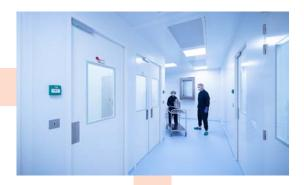
To enter the heart of the manufacturing area where aseptic production takes place, operators enter another personnel airlock where they change from ISO class 7 clothing into sterile, ISO class 6 gowns. The ISO class 6 cleanroom has a separate "airlock in" and "airlock out" for incoming materials, finished goods, and personnel in accordance with the new Annex 1 regulations.
