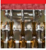
We house two fully automatic filling units for the aseptic filling of organic and volatile solvents and aqueous solutions into ampoules up to 30 ml. This aseptic process is validated by media simulation and executed by a qualified process team. This filling process can be further extended by fully automatic visual inspection, labelling and the positioning of an ampoule breaker.
